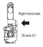
The diagram below shows the S-axis at  $0^{\circ}$  and at  $180^{\circ}$ . This is the configuration when the L-axis and the U-axis are viewed from the righthand side.
