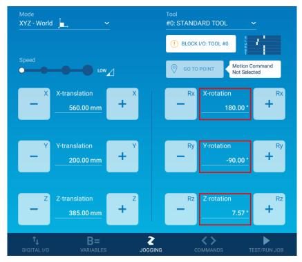
Fig. 2-24: TCP Orientation Panel
