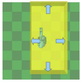
If the {Keep Robot Outside} is selected for Monitor Type, to the walls, move the manipulator toward all the direction where it can make approach and check that it stops just in front of each wall (test each wall).
