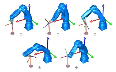
The greater the difference between the five postures, the better. No two recorded postures can match and calibration accuracy will decrease if multiple poses are similar or rotated in a constant direction. Repeating this procedure multiple times may increase the accuracy of the resulting TCP.
