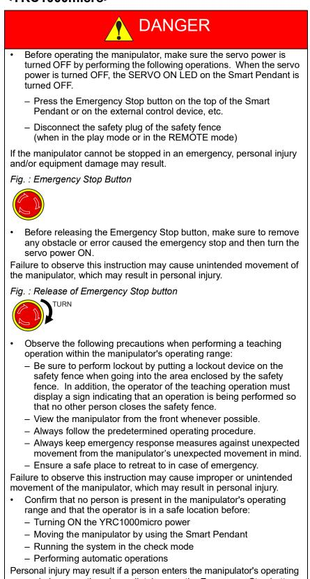
Personal injury may result if a person enters the manipulator's operating range during operation. Immediately press the Emergency Stop button whenever there is a problem. The Emergency Stop button is located on the top of the Smart Pendant.
