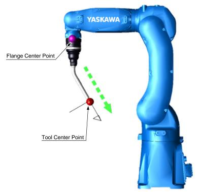
When "0" is set to the speed limit, it becomes the stop position monitoring. the stop position monitoring is performed to TCP or FCP to confirm each point does not move.
