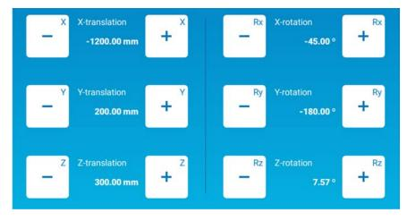
The tool coordinates are defined at the tip of the tool, assuming the effective direction of the tool mounted on the manipulator's tool flange is the Z-axis. Therefore, the tool coordinates axis direction moves with the wrist.
