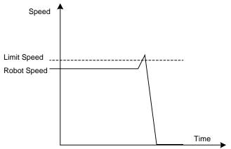
Along with the above-mentioned monitoring, when it is in the MANUAL (TEACH) mode, the speed is always monitored to be 250 mm/sec as the MANUAL (TEACH) mode safety speed.
