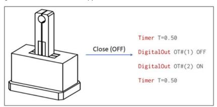
Similarly, opening the gripper might have the inverse logic (turn ON Output #1 and OFF Output #2)
