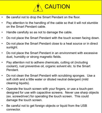
Do not connect the Smart Pendant to except for the YRC Controller.
