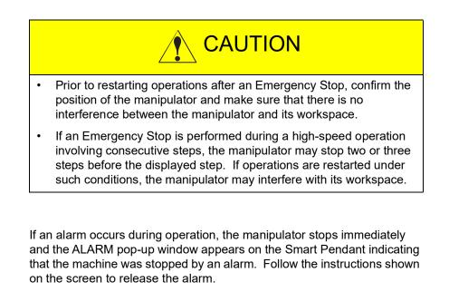
To display the ALARM pop-up window again during alarm occurrence, press the Alarm icon on the status bar. To view previous alarms that are currently inactive, select {ALARM HISTORY} under {MENU}.
