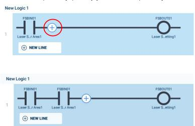
Or, press input relay, then press {+} on the input relay. New input relay will be added at the corresponding position.
