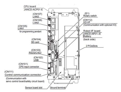
Fig. 12-2: YRC1000micro (LAN Connector)
