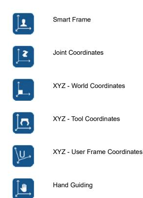
Jogging Mode can be switched in MANUAL (TEACH) mode for Joint Coordinates, XYZ World Coordinates, and XYZ Tool Coordinates by pressing this button. XYZ User Frame Coordinates requires a User Frame be defined to select. Hand Guiding and Smart Frame cannot be selected via the Status Bar. They can be selected on the Robot Jog panel.
