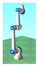
HC10 Torque Calibration Pos. 2 (U-axis: 180 degrees)
