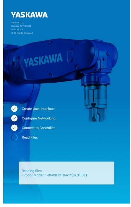
In case the Smart Pendant does not complete the startup sequence due to an error, such as YRC Controller incompatibility, an {Export Logs...} will appear. This button can be used to save internal logs to a USB storage device to aid troubleshooting by a YASKAWA Representative.
