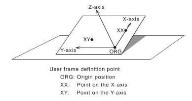
ORG is the origin position. XX is a point on the X-axis. XY is a point on the Y-axis side of the taught user coordinates. The directions of the Y- and Z-axes are determined by point XY.
