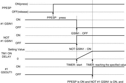
PPESP is ON and NOT #1 GSIN1 is ON, and ON DELAY TIM1 reaches the specified value so that #1 GSOUT1 is ON
