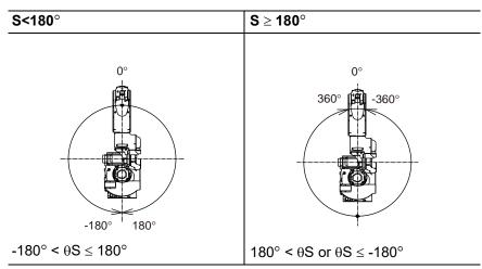
Note that  $\theta S$  is the angle when the S-axis home position is  $0^{\circ}$ .
