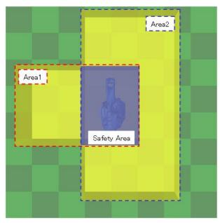
*Fig. 11-7: Simultaneous Monitoring: Multiple Areas (Inside the Monitoring Area + Outside the Monitoring Area)*
