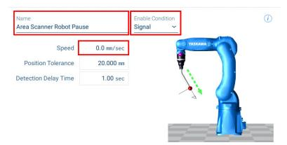
After changing the Enable condition to Signal, the "Advanced Settings" screen will pop-up and you can select a signal for your "Setting Activation Signal" drop-down.
