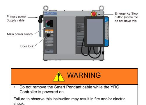
Fig. 1-4: YRC1000 Front View with Smart Pendant
