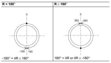
Note that  $\theta R$  is the angle when the R-axis home position is  $0^{\circ}$ .
