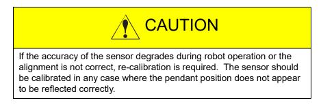
To calibrate, the operator holding the pendant should stand facing the front of the robot and press the {CALIBRATE}. The calibration procedure can be repeated at any time if the robot TCP motion does not reflect the operator's physical position.
