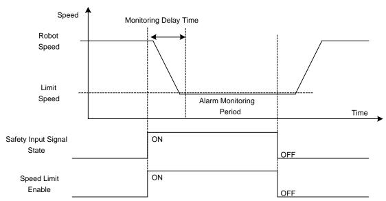
In case an abnormality is detected, the power supply to the motor is stopped using the machine safety, and alarm is notified. Press reset button on the alarm notification once the abnormality is solved.
