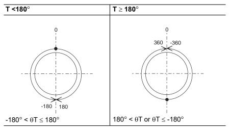
Note that  $\theta T$  is the angle when the T-axis home position is  $0^{\circ}$ .
