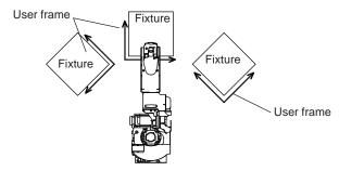
When performing arranging or stacking operations, the incremental value for the parallel shift is easily set by setting the user frame on a pallet.
