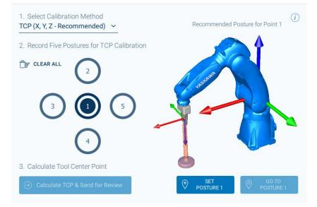
A dialog may appear if the active tool does not match the Tool selected from the list. These must match to accurately perform the TCP calibration procedure.
