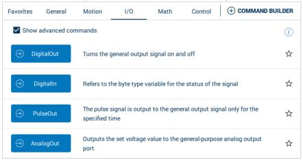
Toggle the general purpose output signal ON/OFF from the {I/O screen} (refer to *chapter 7.4.2.2 "I/O Screens*" for more information)
