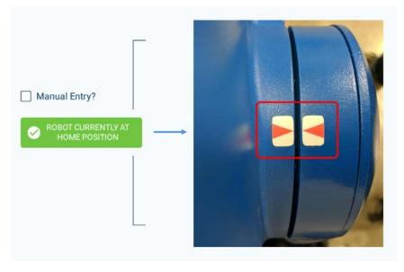
In the case of arrow misalignment for one or multiple axes, Home Position Calibration is required. The following sections discuss how to perform the calibration.
