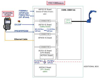
In YRC1000, for the connection of the General Purpose Safety I/O board (Option), either the board of JANCD-ASF02-E (8 points available) or JANCD-ASU03-E(16 points available) can be connected to each safety circuit board (JANCD-ASF01-E).
