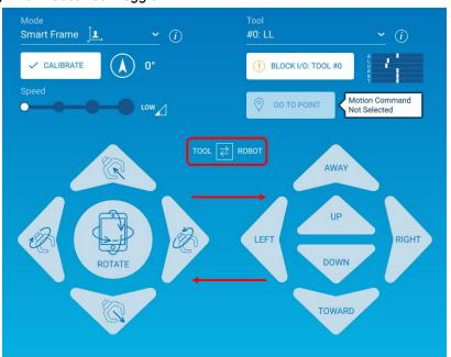
Additionally, the membrane [Jog Keys] can be used for Joint Axis jogging in Smart Frame Mode.
