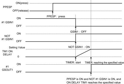
ON DELAY TIM1 reaches the specifie so that #1 GSOUT1 is ON
